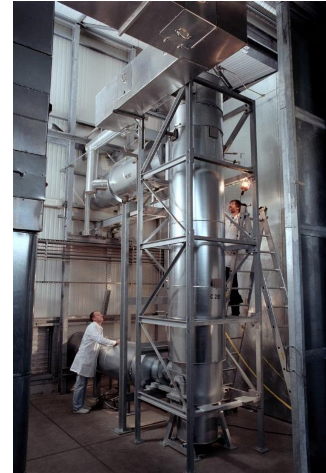
Part of the SCWG pilot plant at KIT, 100kg/h
