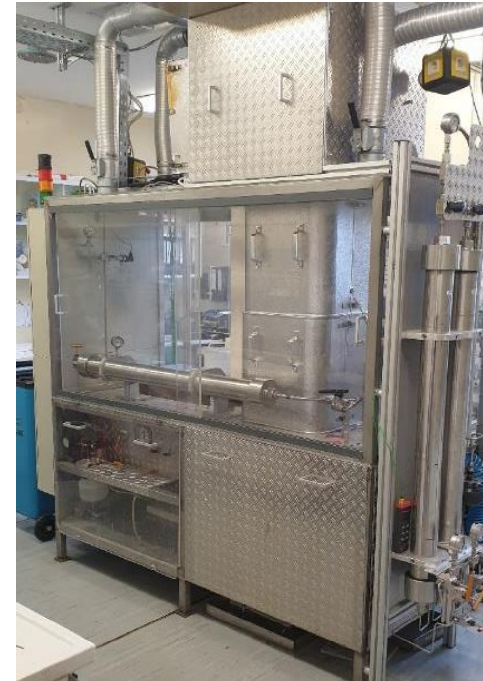
SCWG laboratory plant at KIT, 1 kg/h
