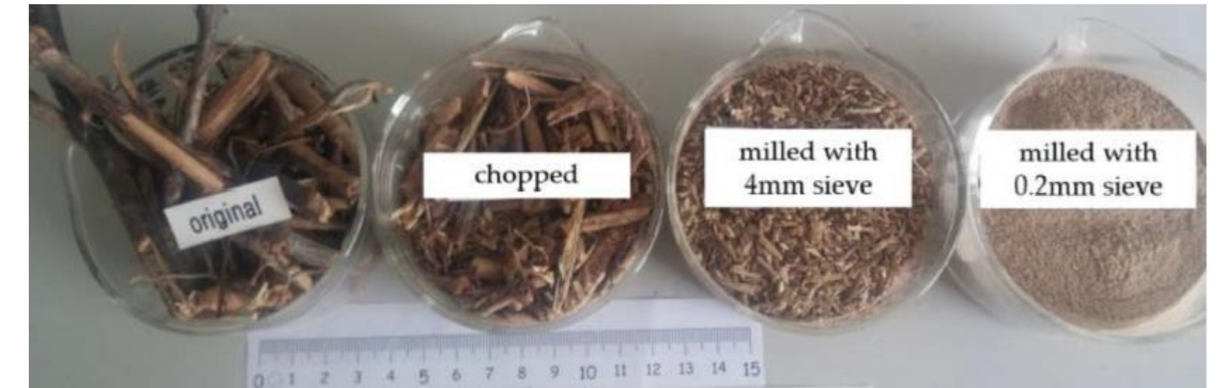
Size reduction of biomass for creation of biomass slurry
